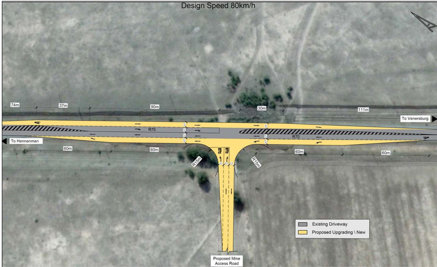
Figure 5. Required upgrades to the R70 and mine access intersection
